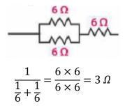
The third resistor is in series, so the equivalent resistance is calculated as;
