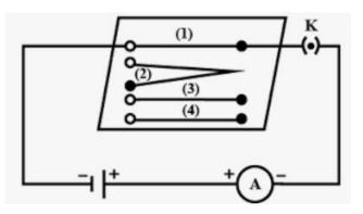
At point plug the key and note the current in ammeter. Replace the nichrome wire by another nichrome wire of same thickness but twice the length that is 2t at point 2. Again, note the reading. Now, replace the wire by a thicker nichrome wire of same length I (marked 3). A thicker wire has a larger cross-sectional area.
