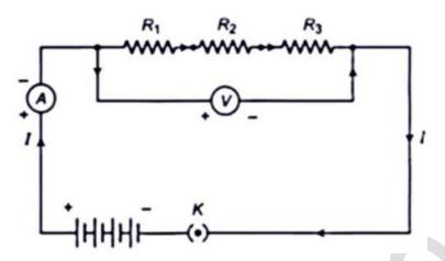
The key K is closed and the ammeter reading is recorded. Now, the position of ammeter is changed in between the resistance again, the ammeter reading is recorded each time, there was identical reading each time, which shows that same current flows through every part of the circuit containing three resistance in series connected to a battery.
