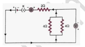
The resistance of parallel combination of two resistors (4  $\Omega$  each) is 2  $\Omega$ .
