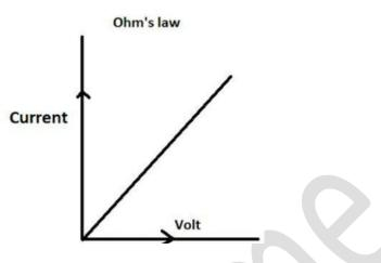
Ohm's law is not good under all conditions as it is not a fundamental law of nature. It is obeyed by metallic conductors only when physical conditions like temperature etc. are kept unchanged. It is not obeyed by a lamp filament, junction diode, thermistor etc. called non-ohmic conductor.
