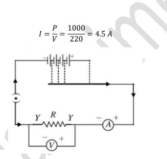
So, the rating of fuse-wire is 5 A which is greater than 4.5 A.
