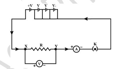
A battery of 4 cells resistance wire, A an Ammeter and V a Voltmeter.
