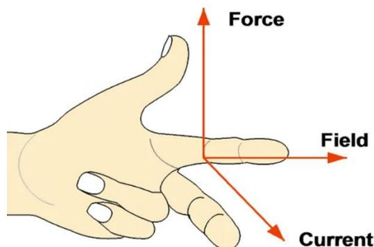
Fleming's left-hand rule gives the direction of force experience by a current carrying straight conductor placed in an external magnetic field.
