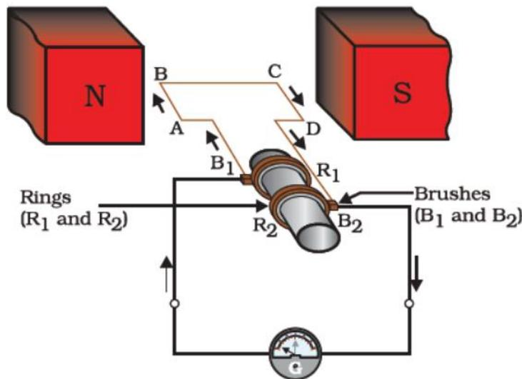
As the coil rotates, the two rings also rotate with the coil. The brushes P and Q keep contact with the rotating ring. When the coil starts rotating with arm AB moving up and CD moving down (clockwise) cutting the magnetic lines. According to Fleming's right-hand rule, the current is induced in these arms in the direction ABCD.
