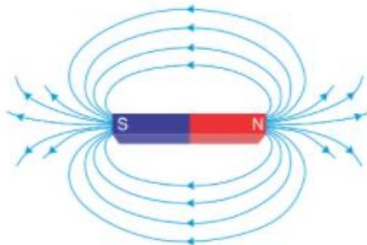
**Magnetic field lines around a magnet bar**
