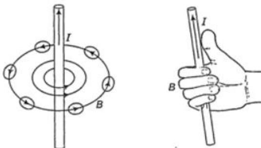
The deflection of the compass increases because the magnetic field  $B$  due to current carrying straight conductor is directly proportional to the strength of the current  $I$  passing through it.
